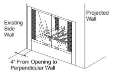
Figure 2 - Typical Two-Sided Fireplace Installation
